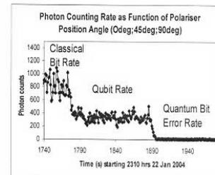
Fig. 1: Linearly polarised single-photon pulse counting rates: B92 protocol single-channel quantum key simulation over 26 km path.
