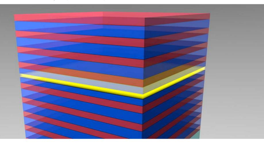
This thin polymer film is approximately 35 nanometers thick, for comparison a sheet of paper is about 100,000 nanometers thick. The bosonic particles are created through interaction of the polymer material and light which bounces back and forth between the two mirrors.
