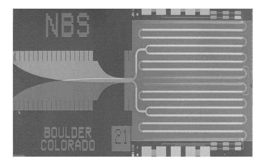
Chip-sized one-volt voltage standard device used for standards measurement. It was developed by NIST based on an array of 3020 superconducting Josephson junctions.
