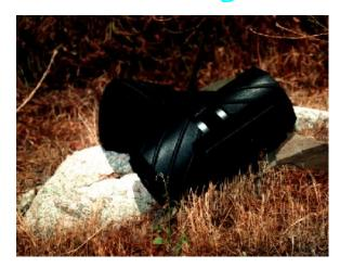
Unique All Surface Drive<sup>m</sup> 90 percent of the vehicle's surface rotates around the machine for maximum traction over all terrain...
