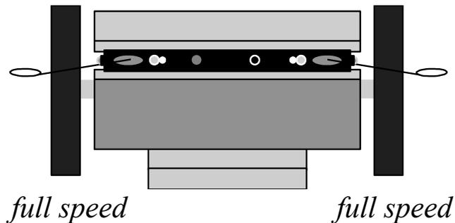
Observe: both wheels rotate in the forward direction and at the same speed.
