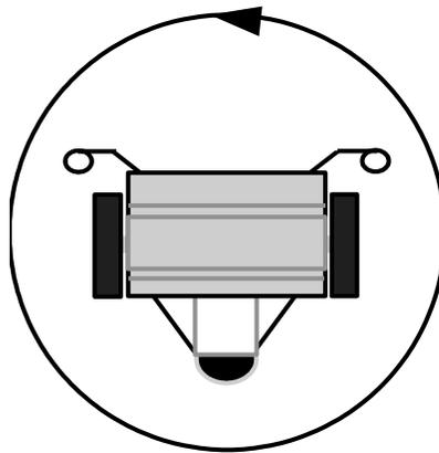
*Observe: the right wheel is turning forward and the left wheel is turning backwards.*
