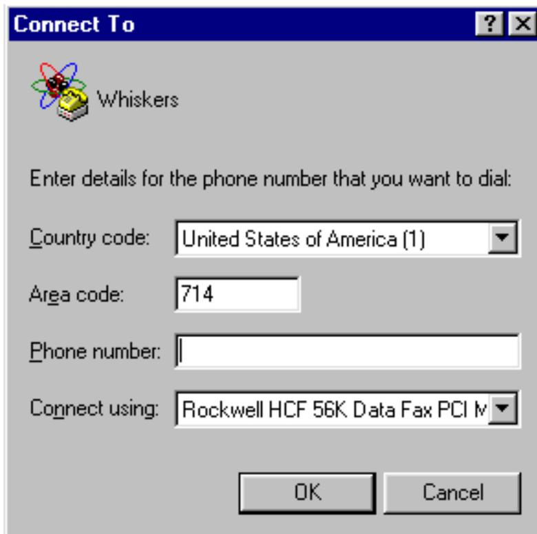
5) Click on Connect using: and choose either Com1 or Com2 depending on the physical port you have the Whiskers cable connected to then click on OK...
