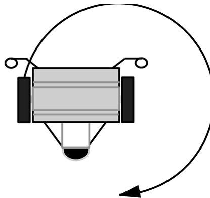
*Observe: the robot rotates 3/4 of the way about the right wheel.*
