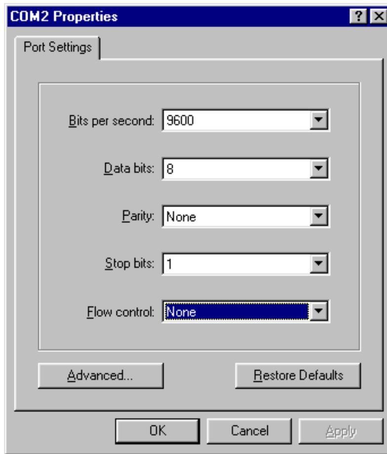
7). You will now be at the screen below...plug the cable into the serial port on your computer if it hasn't already been done and turn the robot on...
