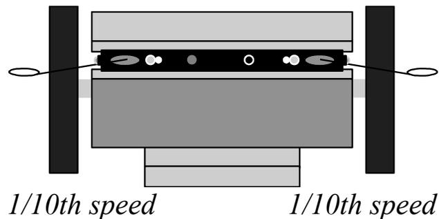
*Observe: the wheels slowed down. This is caused by our use of the **SAVE-SPEEDS** word earlier and Whiskers<sup>tm</sup> remembered the previous speeds.*
