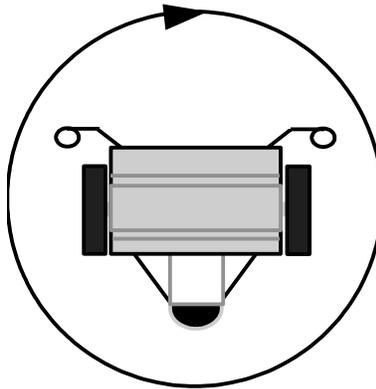
*Observe: the left wheel is turning forward and the right wheel is turning backwards.*
