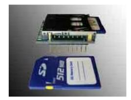
The DOSonCHIP SD/MMC Module integrates the CD17B10 silicon and SD/MMC socket onto a simple drop-in module that is easily added to an embedded design. This module has a small 1.2" x 1.6" footprint as it mounts the CD17B10 and its components under the SD/MMC socket. All the features of the CD17B10 are available.
