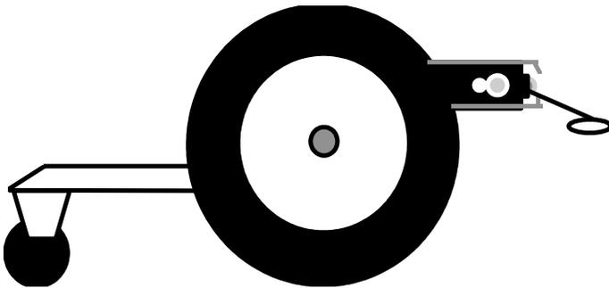
Whisker's is easy to use and fun to program. Whisker's is a three-wheeled, battery-powered, free roaming, obstacle-avoiding robot. His propulsion is provided by two 12 volt DC geared motors. Whiskers has a computer on board which allows you to control and program him. Using simple commands like FORWARD, STOP, and many other english words, you can control him interactively by typing the commands on the computer.
