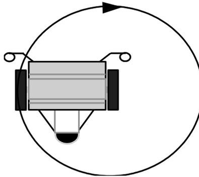
Observe: the left wheel is turning forward with the right wheel stopped.
