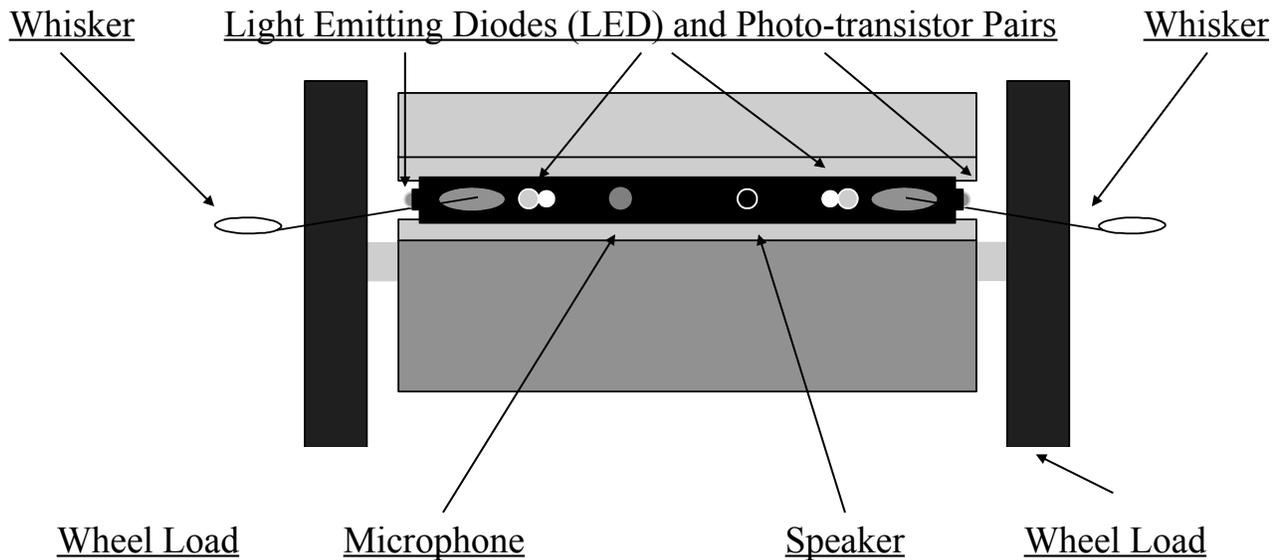
***Touching***-Whiskers on each side give the robot the ability to *feel* objects. This is called a tactile sensor.
