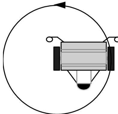
*Observe: the right wheel is turning forward with the left wheel is stopped.*
