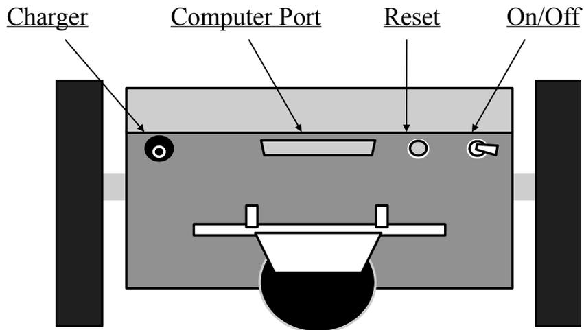
**Charger**-This is Whiskers™ food input. The robot can continuously operate about three to four hours depending on options and the age of the battery. It is a good idea to always keep the Whiskers robot plugged in when not in use so he is well fed and ready to play at any time.
