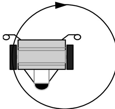
*Observe: the robot rotates 360 degrees about the right wheel.*
