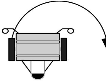
*Observe: the robot rotates 180 degrees about the right wheel.*
