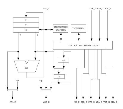
Figure 1: Block Diagram of the S16X4 Processor.
