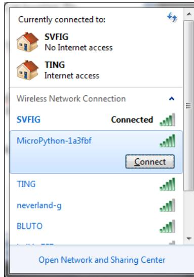
Connect to MicroPython-xxxxxx station, where xxxxxx is the ID of the ESP8266 chip. You will be asked to enter a password to connect. Type in the universal password for NodeMCU: 'micropythonN', ending with a capitalized N.
